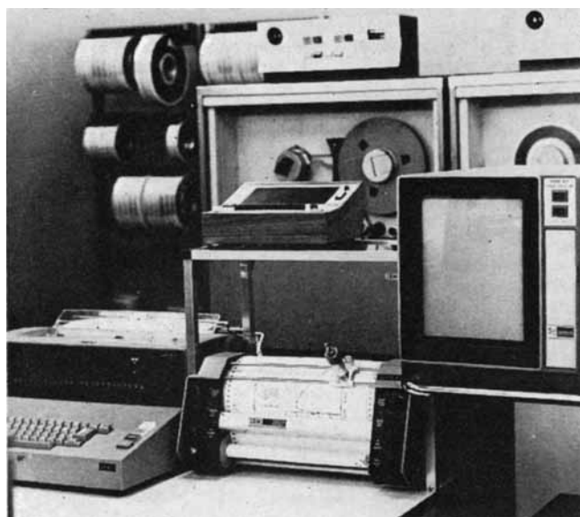
Figure 2—Keyboard entry device, incremental plotter, and visual display console used in connection with the IBM-1800 computer.
